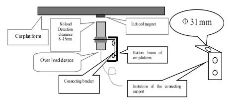
Attention: The system connecting support should be prepared by the customer according to the concrete condition.
