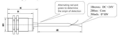
**Attention :** Output wire of this device must not be connected with external power supply to avoid everlasting damage. The company is not responsible for the resulting damage.
