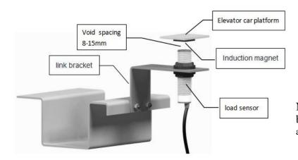
Note: The system connection bracket requires the user to make it according to the specific situation.
