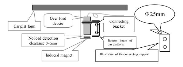
Attention: The system connecting support should be prepared by the customer according to the concrete condition.
