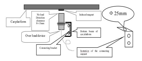
Attention: The system connecting support should be prepared by the customer according to the concrete condition.
