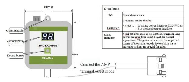
Note: All wiring ports are strictly prohibited from plugging and unplugging; Do not connect the power cord to the CAN communication port (port P/N), otherwise the device will be damaged immediately!
