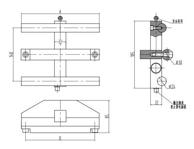
Note: ø6 wire rope must be used to connect the safety ring and secure it on the support of the traction machine to prevent the sensor from falling off during the installation and commissioning of the elevator to ensure personal safety
