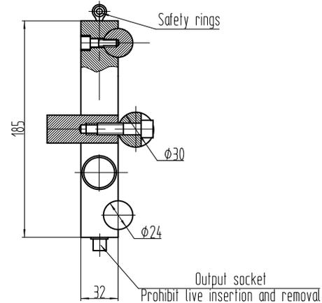
Note: the installation must use  $\phi 6$  wire rope link safety ring and solid in the tractor nail to prevent the elevator installation and commissioning when the sensor off, to confirm personal safety.
