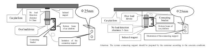
Attention: The system connecting support should be prepared by the customer according to the concrete co
