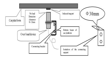
Attention: The system connecting support should be prepared by the customer according to the concrete condition.
